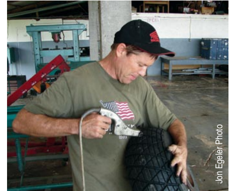
Mark Friesen using the special tool to cross-hatch a new CE 206 tire. The completed job appears as though it were a factory job!
