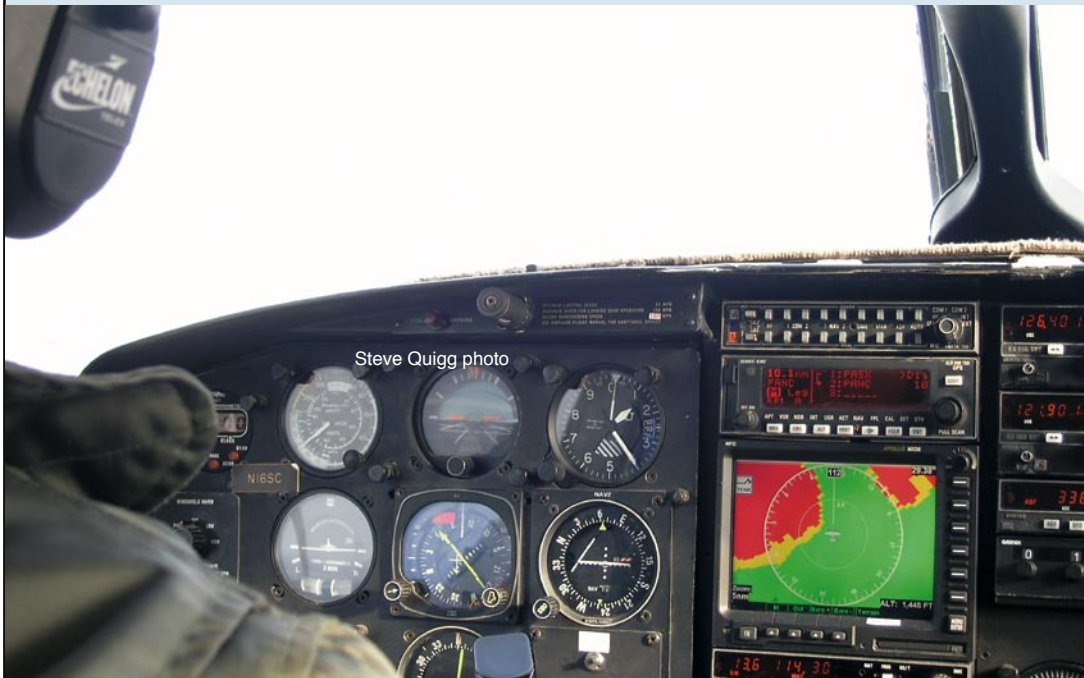
Capstone at work! Note the view in the MFD. The airplane is in the center of the screen over the green area. The mountains are just to the left, represented by the red area. Though the pilot can’t see anything out the window, he knows precisely where he is and that he is in no danger of a controlled flight into terrain (CFIT) accident.
